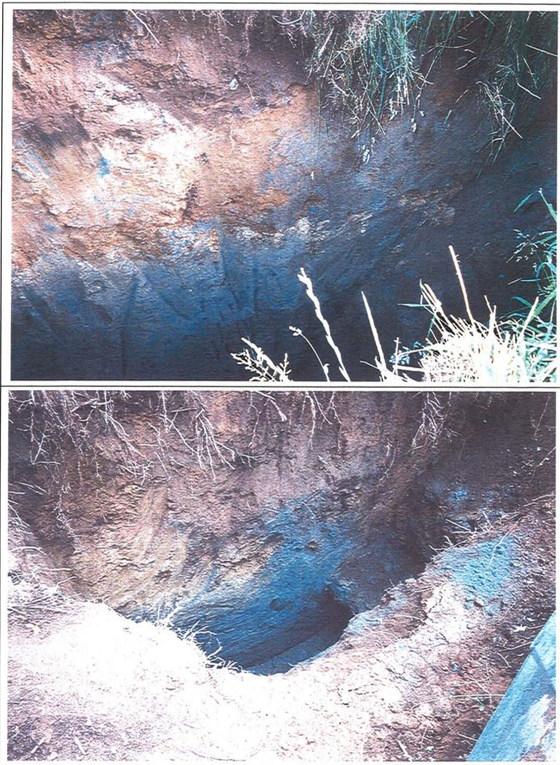
Woodtrails - Supplemental test pits in detention pond. Dense to very dense Silt and Silt with Gravel. Excavated to 20 feet.
